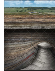
SD4 - Natural Gas Trap Against a Salt Dome
